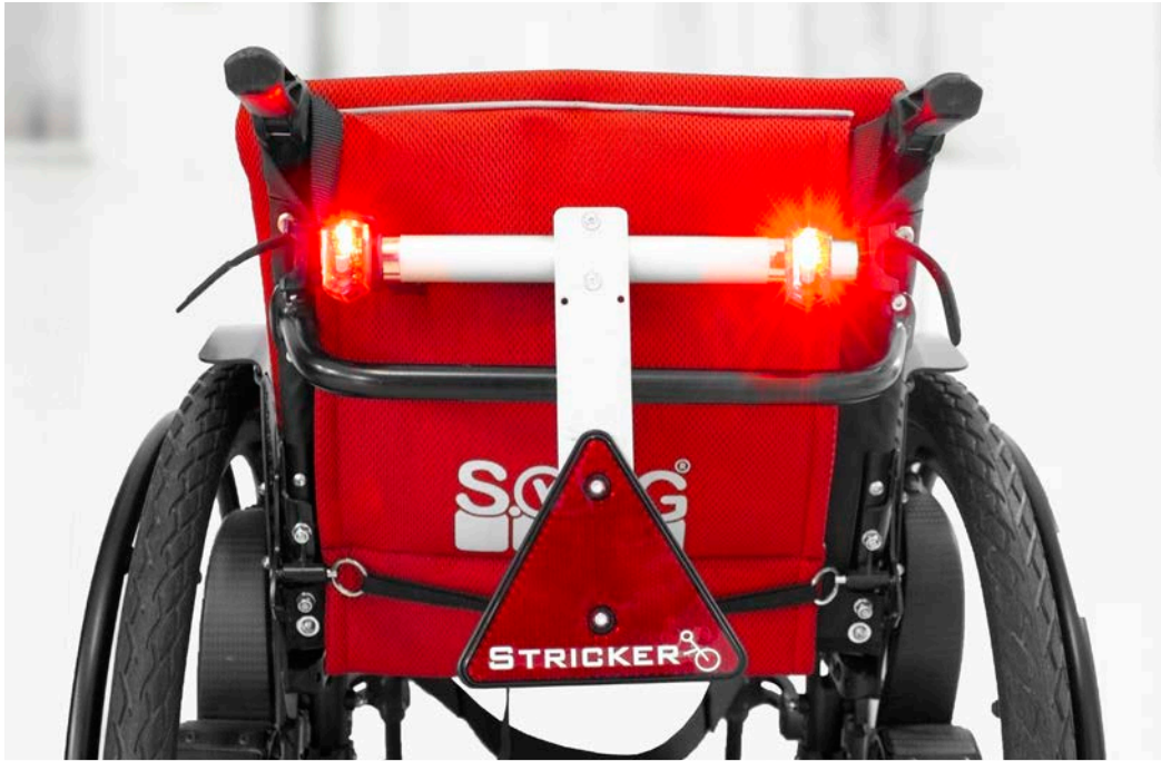
Tail light bar with battery-powered tail light and warning triangle
