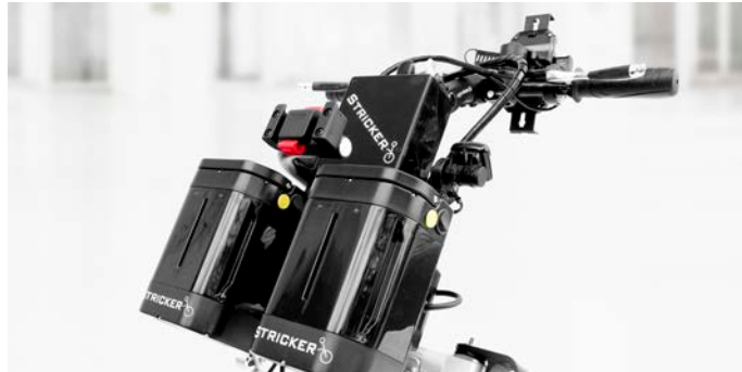
Lipo Lomo - two battery holders on the head tube
