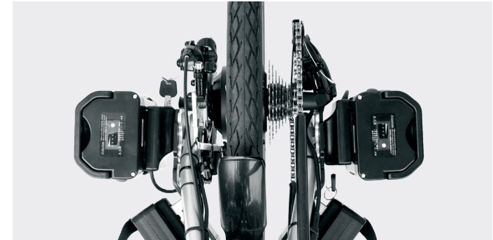
Lipo Smart - two battery holders on the fork
