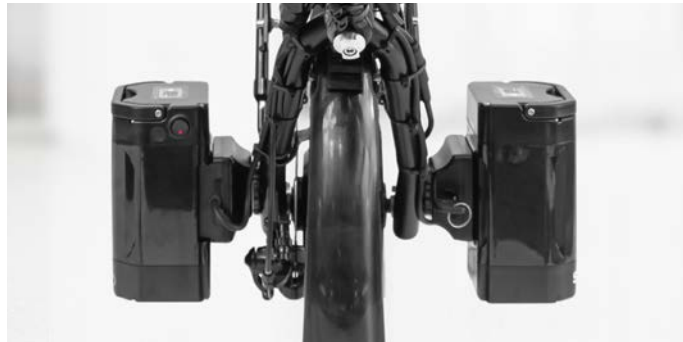
Lipo Lomo - two battery holders on the fork
